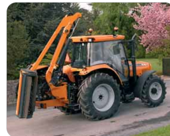
Above: Integrated Active Transport Control reduces shock loads and gives faster, safer transport of linkage-mounted equipment
