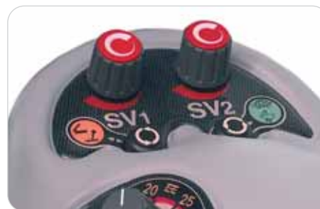
SV1/SV2 Speed memories, Dyna-VT operating modes and range selection all in one convenient 'pod'
