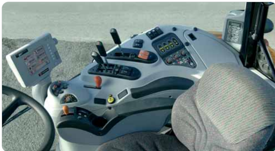
SV1/SV2 Speed memories, Dyna-VT operating modes and range selection all in one convenient 'pod'
