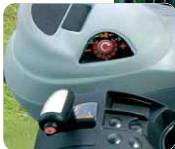
Right-hand controls include the 'T-handle' gear lever with a push-button for range selection and the power shuttle Comfort Control switch
