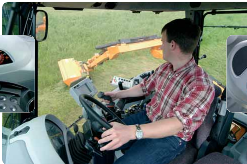
Right-hand controls include the 'T-handle' gear lever with a push-button for range selection and the power shuttle Comfort Control switch
