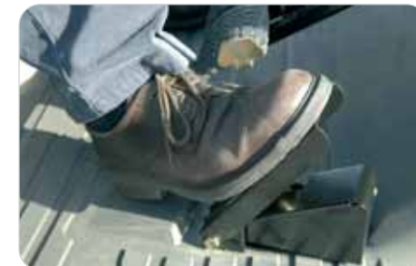
Pedal mode offers precise forward speed control, regardless of engine speed.
