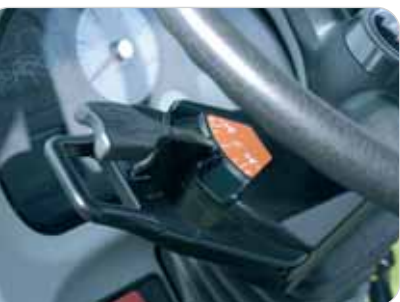
Left-hand Power Control (above) leaves the right hand free to operate implement controls and other functions
